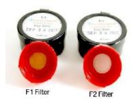
The instrument uses two filters to eliminate the signal caused by interfering substances. Measurement is first made with a filter to determine the background level. A second filter will allow the meter to subtract the background and give the formaldehyde vapor concentration without interference.
