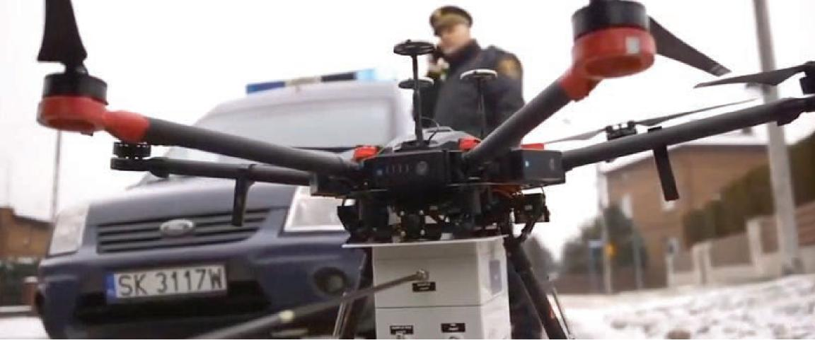
The Scentroid DR1000 flying laboratory provides continuous monitoring of multiple chemicals. While in flight, five built-in chemical sensors can provide remote monitoring of chemicals selected at the time of ordering. The Scentroid DR1000 can be used to sample and analyze ambient air at heights of up to 150 meters above ground level that was previously impossible to accomplish. Air quality mapping, model ver-
