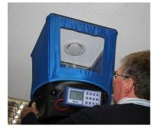
By simply adding the 400 mm x 400 mm short canvas (as illustrated), a starting volume of 5 l/sec, 18 m<sup>3</sup>/hr, 11 cfm is achievable and being only 610 mm high, it gives easy access to the grills. Base Unit Set of Poles Low Volume Adaptor Plate Airflow Straighteners Wheeled Carrying Case
