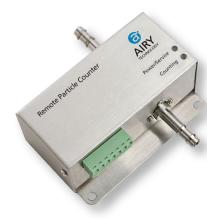
The Airy Technology® P235 Remote Particle Counter measures 0.5 µm and 5.0 µm with a flow rate of 0.1 CFM (2.83 LPM). Integration is easy into a real-time monitoring or building management system via Modbus RTU. The P200 models are the smallest 0.1 CFM remote particle counters on the market and have easy mounting options. The Airy Technology® P235 unit complies with ISO 21501-4 and includes a 1 year limited warranty.
